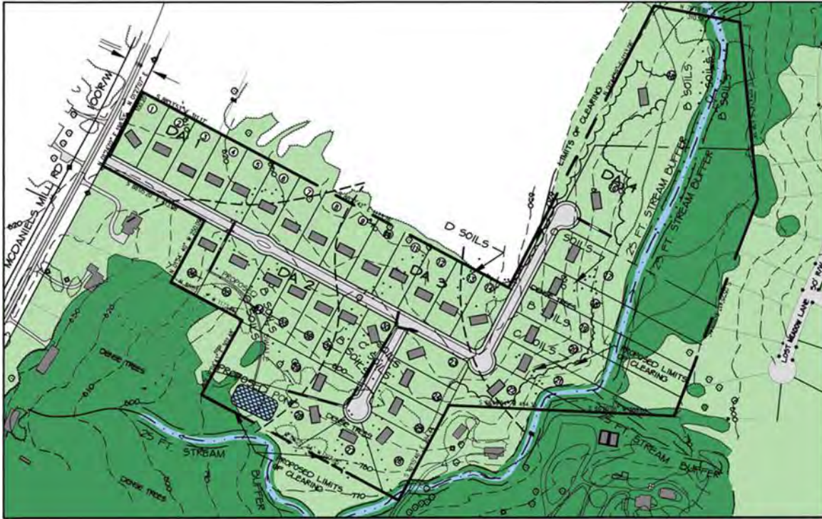
Figure 4-1. Residential Subdivision with Conventional Design and Central Stormwater System
