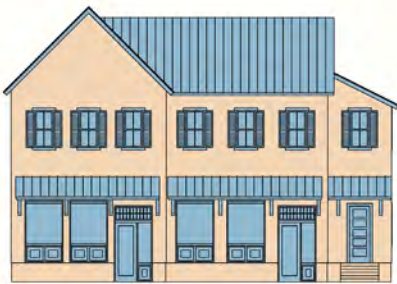
Storefront windows and doors allow pedestrians to see into the ground floor spaces. A stair and elevator tower on the end of the building gives private access to the upper story if desired.
