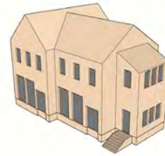
Adding a gable end breaks up the building facade and provides multiple distinct storefronts.
