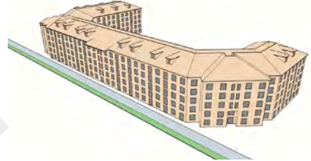
Turning the ends of the building back in to the lot provides a courtyard for parking or building amenities.
