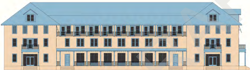
A broad facade is broken up by regularly spaced large windows. The scale of the windows and facade treatment decreases at each level, with the smallest and most residential scale features closest to the top.
