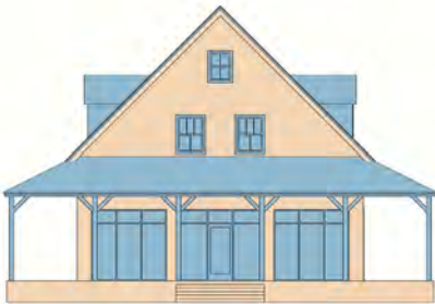
A front facade with storefront glazing and transom windows allows natural light into the lower story space and invites pedestrians in.
