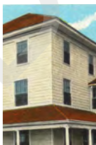
Wood or fiber cement clapboard siding in a variety of colors in whites, grays, earth tones, and pastels are appropriate. Exposures should be 8" or less.
