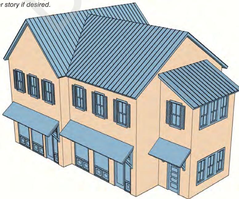
Awnings with brackets and shutters protect the windows from sun and rain.
