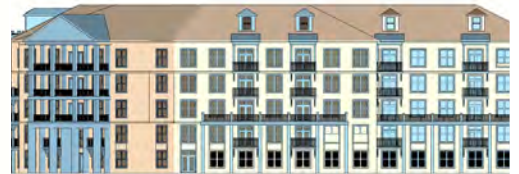
Carrying the same elements of the front facade around the sides creates a coherent building.
