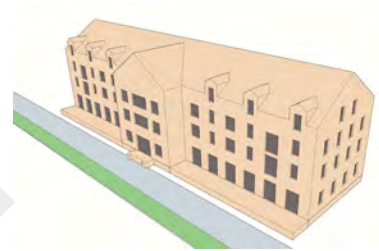
Adding a gable end breaks the facade into multiple masses and makes for a clear point of entry.
