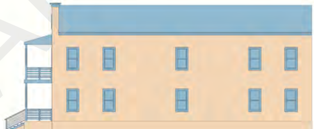
Ground floor side windows are necessary to maintain the visual permeability of the street frontage. Side windows towards the rear of the building are optional, but encouraged.
