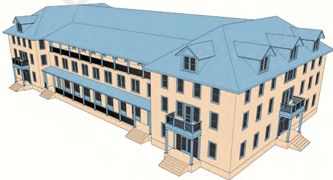
Minimal ornament is needed if the windows and other features are scaled appropriately. Dormers break up the large roof expanses and can be used to bring daylight into loft spaces or to ventilate mechanical spaces.
