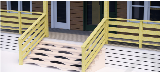
Plank Railing Rustic style of railing with low visibility and horizontal emphasis
