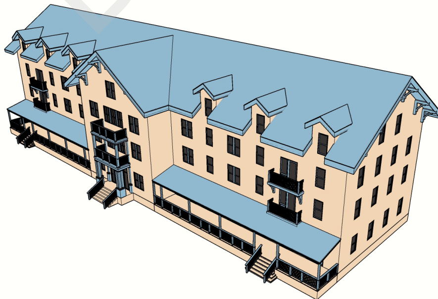
Minimal ornament is needed if the windows and other features are scaled appropriately. Dormers break up the large roof expanses and can be used to bring daylight into loft spaces or to ventilate mechanical spaces.
