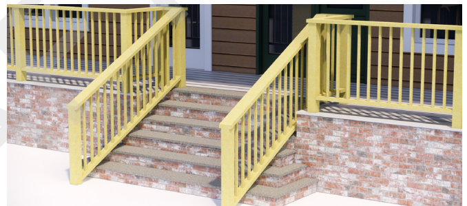
Picket Railing Traditional style of railing with vertical emphasis, picket styles vary
