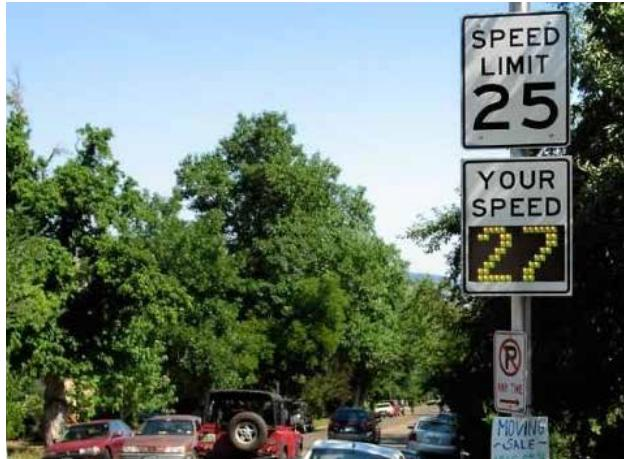
Speed feedback signs can be an effective and low cost tactic to reduce speed along corridors with high pedestrian activity.
