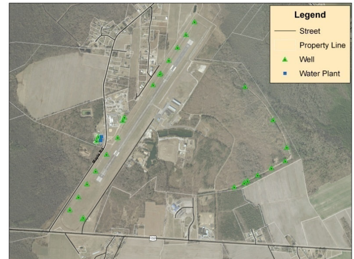
The Well Points Map shows the approximate location of the shallow wells used by the County for potable water usage.
