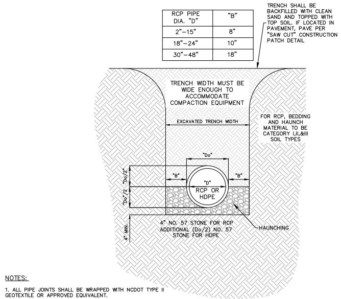
STORM PIPE TRENCH SECTION N.T.S.
