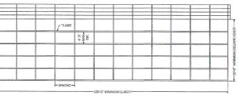
SPACING = 3'-0' FOR WIND SPEEDS BETWEEN 110 MPH AND 140 MPH SPACING = 4°-0" - O4 WIND SPEEDS BETWEEN 140 MPH AND 160 MPI 1 1/2" 18 GA HAT CHANNELS CAN BE USED IN LEU DITYS FOR GIRTS.
