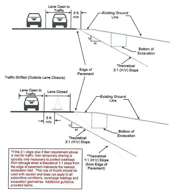
If the 2:1 slope plus 5 feet requirement above is met for traffic, then temporary shoring is typically only necessary to protect roadways from damage when a theoretical 1:1 slope from the edge of pavement intersects the nearest excavation wall. This rule of thumb should be used with caution and does not apply to all subsurface conditions, surcharge loadings and excavation geometries.
