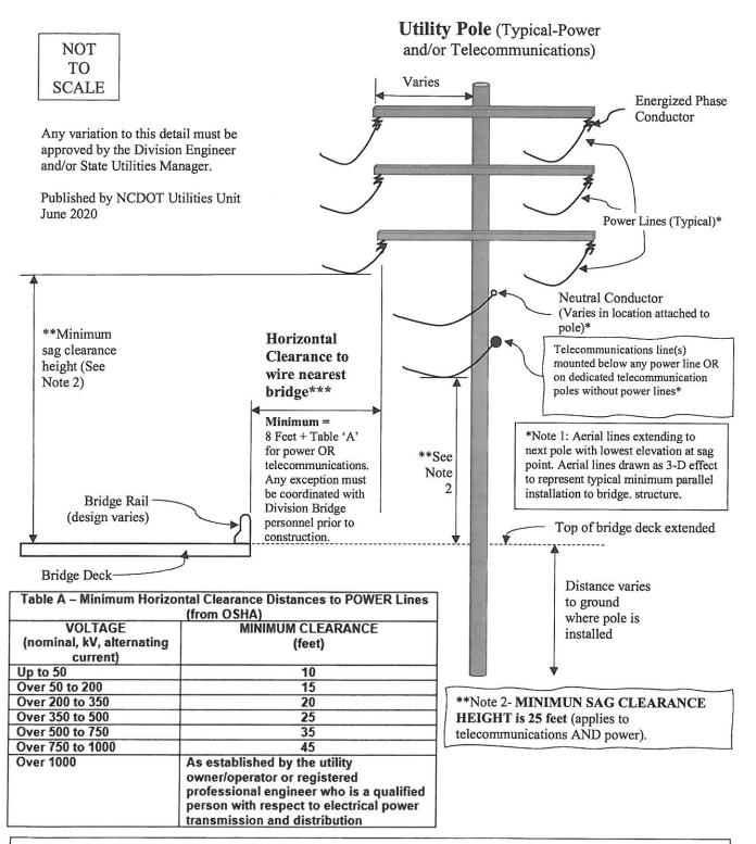
\*\*\*Note 3: HORIZONTAL CLEARANCE EXCEPTION. If vertical sag clearance height for power above bridge deck is ≥ 45 feet AND voltage is ≤ 350kV, then Minimum Horizontal Clearance may be reduced to 3 feet. Any telecommunications attachment to power pole allowed in this exception must have a minimum 25 feet sag clearance height above bridge deck.
