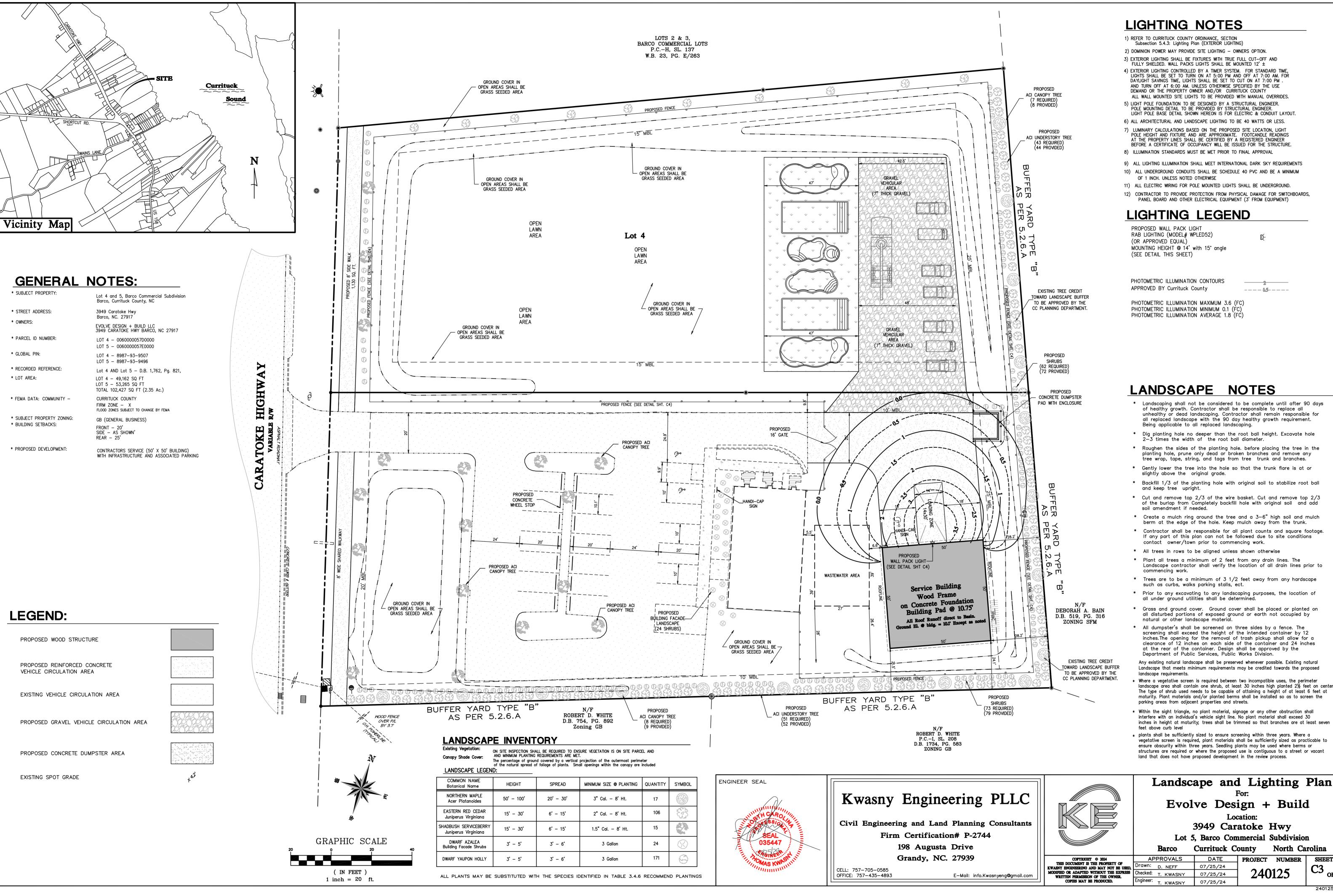
3) EXTERIOR LIGHTING SHALL BE FIXTURES WITH TRUE FULL CUT-OFF AND FULLY SHIELDED. WALL PACKS LIGHTS SHALL BE MOUNTED 12' ±
