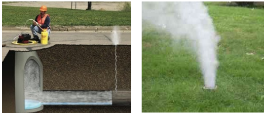
Example of sewer smoke testing
