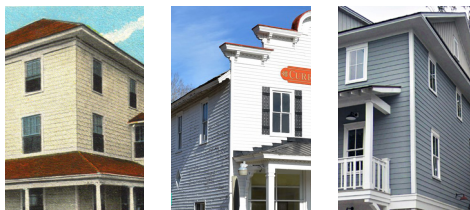
Wood or fiber cement clapboard siding in a variety of colors in whites, grays, earth tones, and pastels are appropriate. Exposures should be 8" or less.
