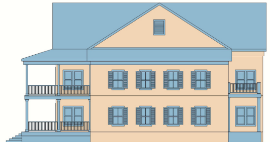
The windows should continue around the perimeter of the building to provide daylighting for all of the interior spaces.
