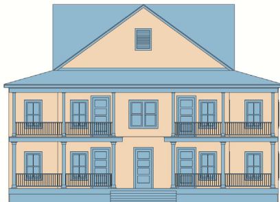
A front facade with doors and generous windows centered on bays is functional and pedestrian friendly.
