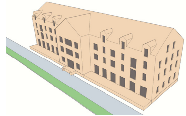
Adding a gable end breaks the facade into multiple masses and makes for a clear point of entry.
