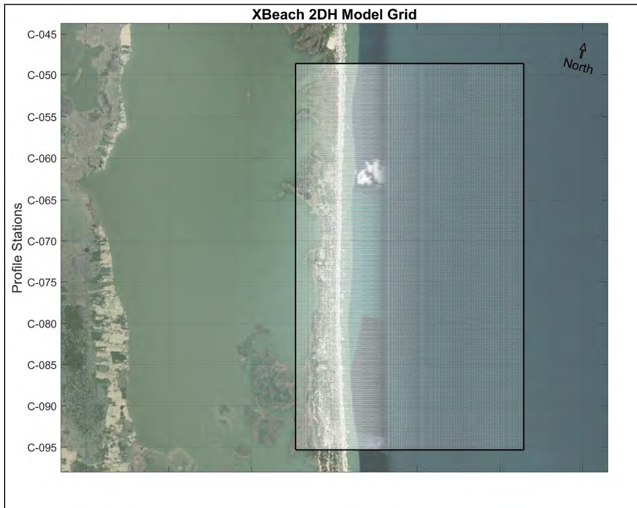
Figure 56. XBeach 2D computational grid showing the model domain extent from Station C-048 to C-096.
