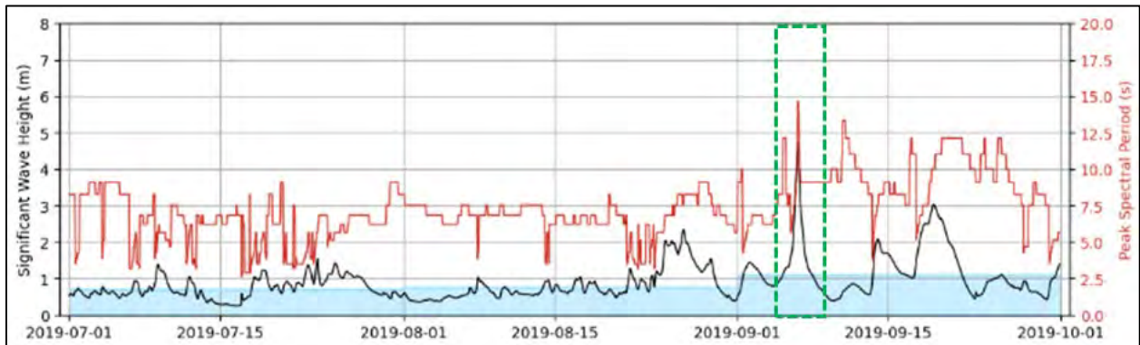
Figure 21. Significant wave height (in black) and peak period (in red) obtained from WIS Station ST63217 for the months of July to September 2019. The green box represents the Hurricane Dorian (2019) timeframe. Source: https://wisportal.erdc.dren.mil/ .
