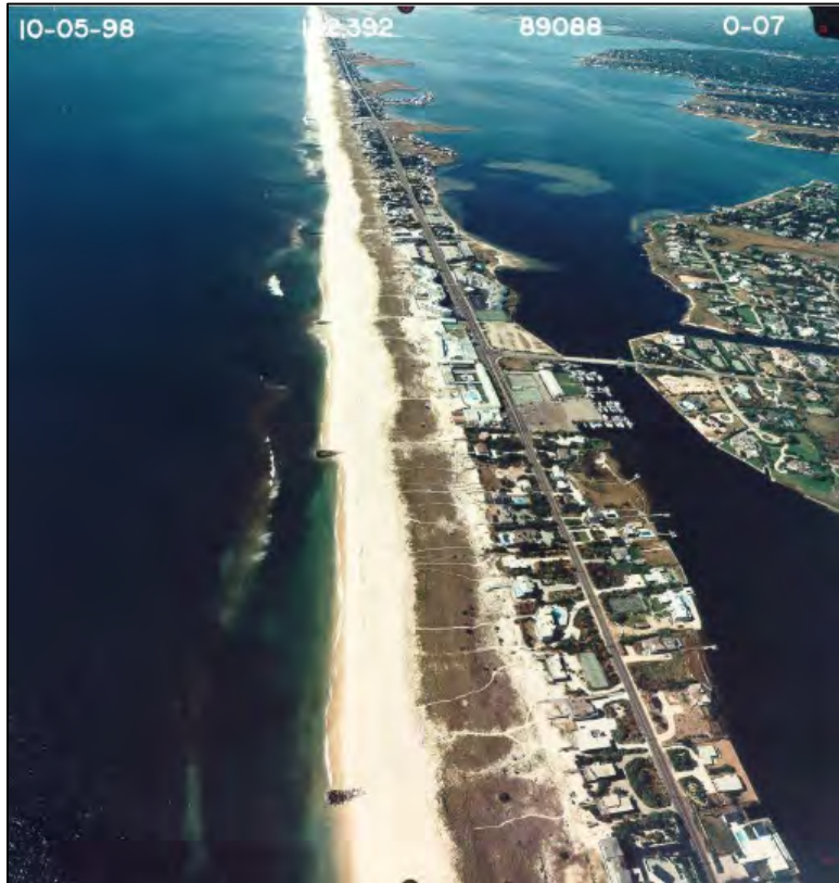
Figure 89. Example of groin field and renourished beach at Westhampton Beach, New York, 1998 (Courtesy USAED, New York).
