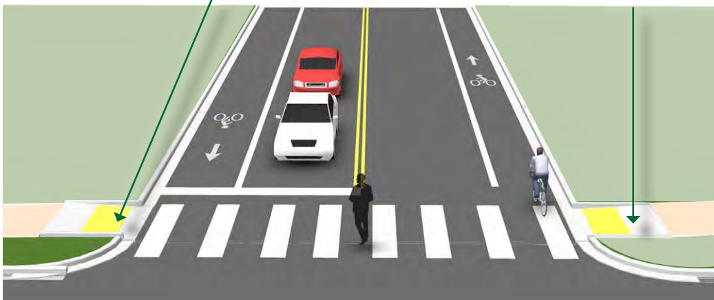
Crosswalk markings legally establish midblock pedestrian crossing
