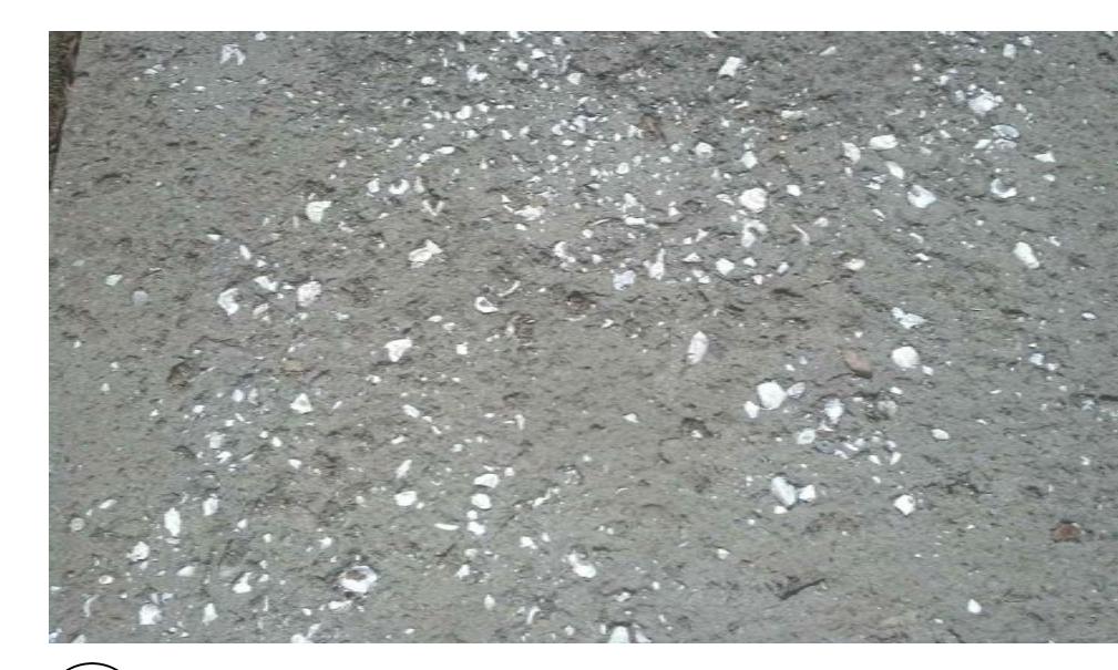
1A CONCRETE TYPE A / SEEDED SHELL AGGREGATE
