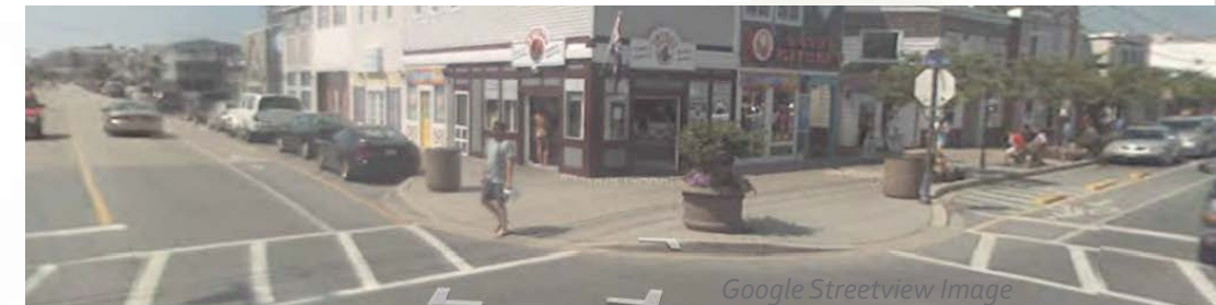
Safety improvements shown here in Bethany Beach include curb bulbouts, crosswalks, and bike lanes.
