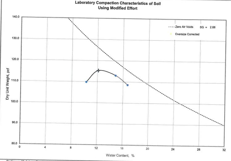
**Optimum Moisture Content** 12.1 Preparation ASTM dry preparation method **Maximum Dry Unit Weight** 115.3 pcf Type of rammer Manual - 10lbf (44.5N) Test Specfication / Method ASTM D1557-12e1-method C Specific gravity - D854 water pycnometer 2.68 Historical Cumulative material retained on: 3/4 in. sieve 3.4 % Coarse Aggregate Specific Gravity -2.68 3/8 in. sieve % #4 sieve % Nat. Plasticity Soil Description Liquid Limit %< #200 USCS
