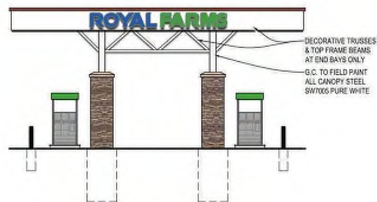
Fuel Canopy - Side Elevation 1/8" = 1'-0"
